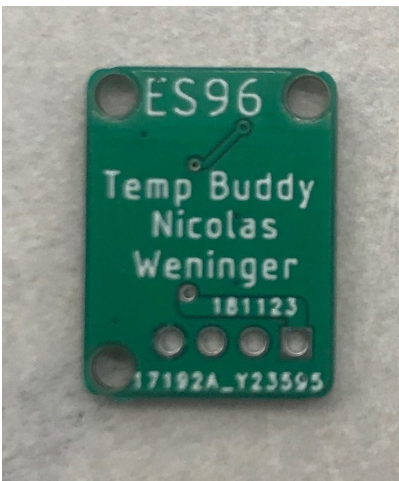
Figure XX: The unpopulated Temperature Sensor Buddy Board rear
