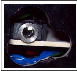
Image 4.12 - Enlarged Download Socket Hole
