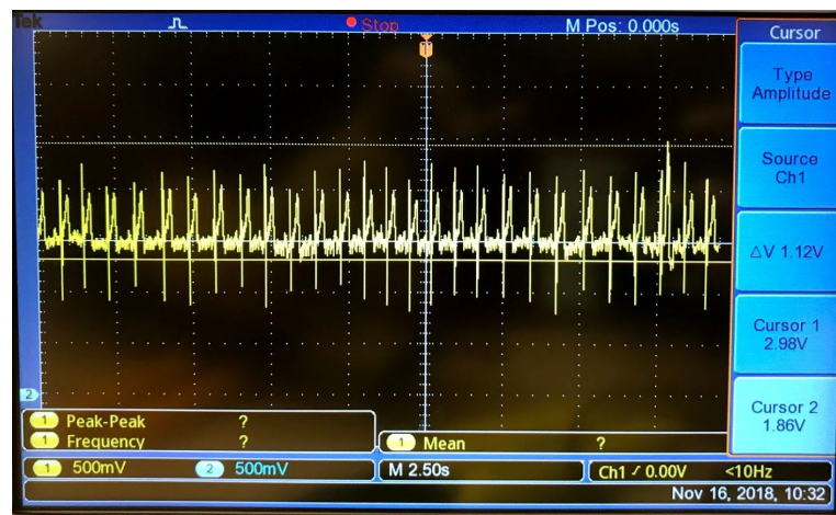
Figure 3.6: ECG signal recorded at the left clavicle (Location II). Note that the signal is quite noisy and has smaller amplitude peaks.
