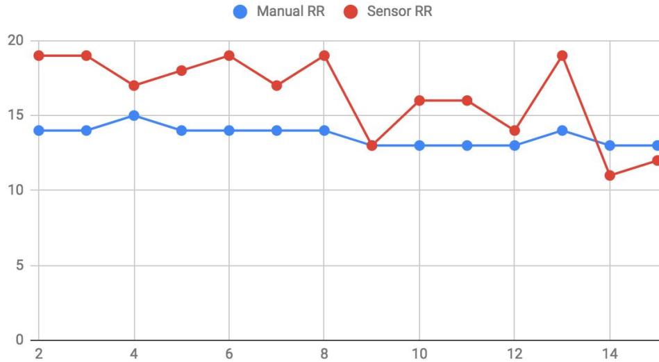
Figure 3.13: Representative graph for one subject of manual respiratory rate (blue) as compared to sensor-determined respiratory rate (red) over 15 trials of 60 seconds total.
