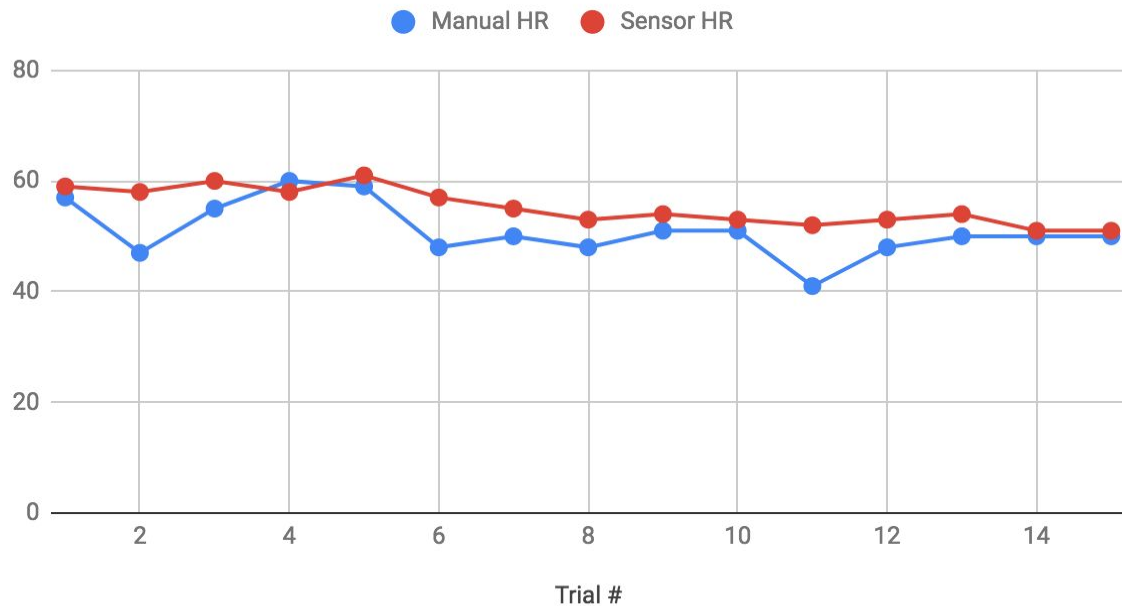
Figure 3.11. Representative graph for one subject of manual heart rate (blue) as compared to sensor-determined heart rate (red) over 15 trials of 60 seconds total.
