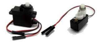
This motor is in a form factor similar to that of a miniature servo, and has an integrated gearbox. Although tests showed it had sufficient torque and speed despite consuming a relatively small amount of power; it did not fit well in our proposed design. In addition, because it used plastic gears, testing showed it would not survive multiple stalls or heavy loading which could have occured during testing. We did not choose this motor.
