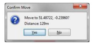
This displays the longitude and latitude the rover will move to, and the distance from its current position. After the user confirms, the target position is changed, and an update sent to the rover.
