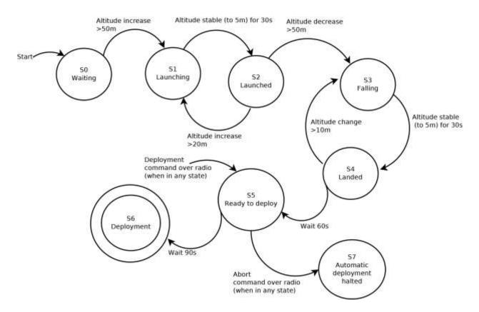
Many stages are required in order to result in an automatic deployment, to prevent false positives accidently deploying the rover. In addition, a 90-second warning will be given over radio before automatic deployment, with the ability to send a command over radio to abort deployment if it is not safe to do so (i.e. it has not yet landed).
