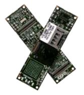
The Gumstix Overo, pictured above, is a small 'computer-on-module' that runs Linux on an OMAP3 ARM processor. We used the TidalSTORM variety, which has 1GB of RAM, a DSP and hardware video acceleration. The combination of a large amount of RAM and hardware video means that we can stream video efficiently, reliably and with surplus CPU power for the other control functionality.
