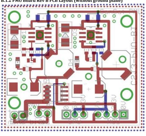
B.1.2 PMU Board Rev B PCB Layout (without ground plane)
