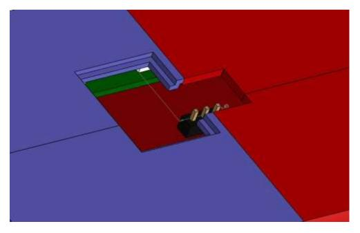
Both holes also have a 1mm rim around their edges, which would allow for a 1 mm acrylic plastic covering, should it have been deemed necessary. A mouldable polymer - such as "Polymorph" could have also been used to serve this purpose.
