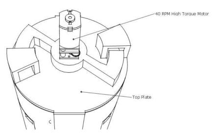
2.5.2.3 Latch Mechanism As mentioned in an earlier section, each side shell has been designed specifically to integrate a "hook" into the top of the part. On the top plate of the overall landing module (and can) a latch mechanism, driven by a 40 RPM high torque motor identical to the one used in the rover to supply the drive, has been integrated. It is made from
