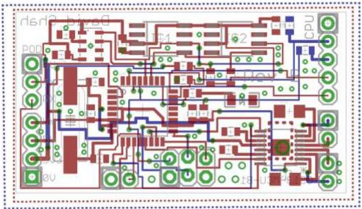
**B.3.2 MCU Board Rev B PCB Layout (without ground plane)**
