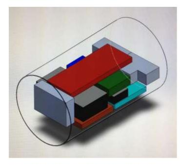
Following the PCB revision, significantly more space was made available, due to the altered dimensions of the PCBs. Overall, all PCBs were made smaller, other than the CPU board, which was small enough and complex to assemble, due to fine pitch components, so did not justify a redesign.
