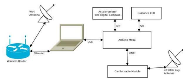
The wireless router is powered off a set of 8 AA batteries, and the Arduino and peripherals are powered from the laptop's USB port.
