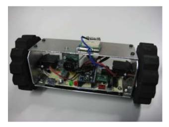
The rover design (above) eventually selected was to place wheels on each side of the CanSat, with an aluminium body between them. This body contained all the electronics, which included a standalone
