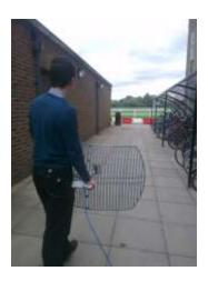
This antenna is highly directional, having a field of view both horizontally and vertically of approximately 10°. Therefore, it was necessary to have some automated or semi-automated system to position the antenna. The initial position, used to establish initial wireless communications, is obtained from the 433MHz RF link to the landing module.
