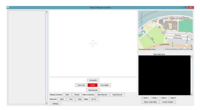
There are a number of parts to our user interface. The pane to the left displays debugging and status messages, for example when a successful landing is detected or when the rover reaches its target position.
