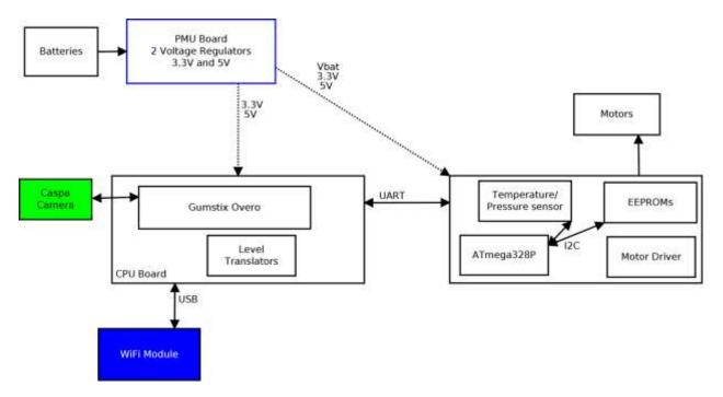
Below is a simplified block diagram of the electronics.
